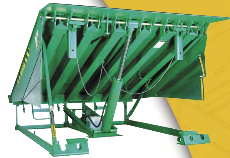
Kelley's HP dockleveler provides automatic hydraulic operation with a single push-button activation and a mechanically activated lip. The HP's unique Gravity-Lip™ automatically extends the lip in a smooth, quiet fashion as the dockleveler descends into the trailer.
