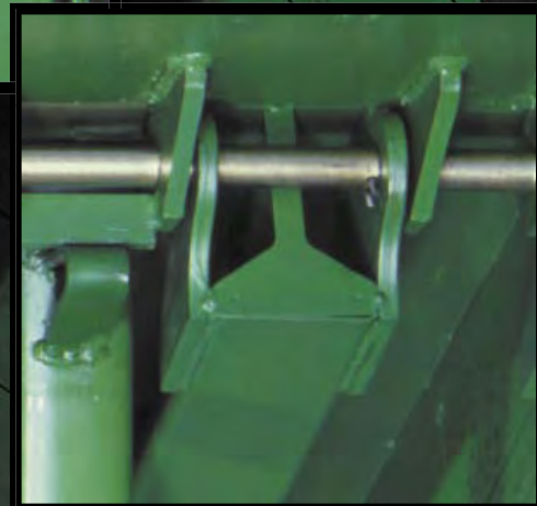
The strength and simplicity of Kelley's exclusive self-cleaning lug-style lip hinge design reduces maintenance and service while prolonging the life of the dockleveler.
